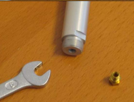
A photograph showing the burner tip assembly with a small silver wrench (SW 6) placed next to it. The brass nozzle has been removed and is lying on the wooden surface next to the wrench. |
